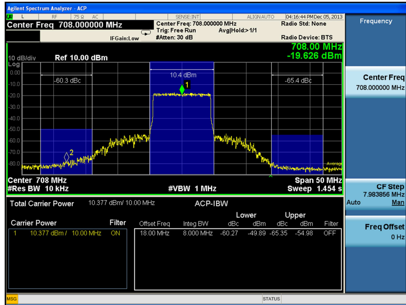
FIGURE 4 Spectrum of IMT UE TM2 signal having an ACLR of 60 dB
