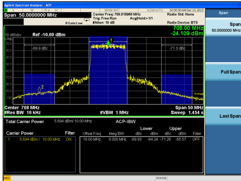
FIGURE 5 Spectrum of IMT UE TM1 signal having an ACLR of 70 dB
